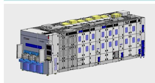
Advanced Wafer Level Packaging (Back-end Assembly Tool)
